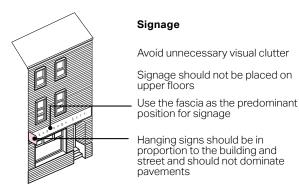
Figure 43: Diagram illustrating well-designed shopfronts.
